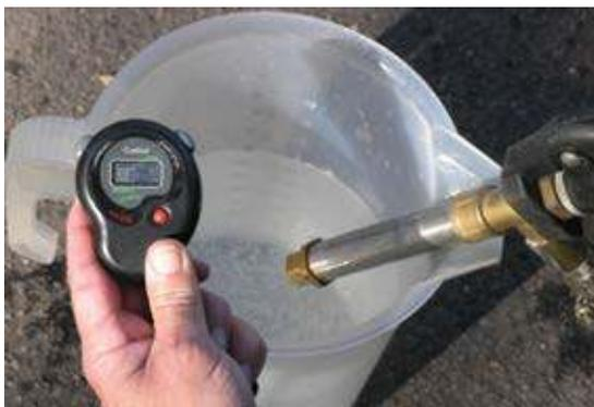
Step 1: Using water, measure how many litres are emitted into a measuring jug from the sprayer in one minute. This is the nozzle output.
