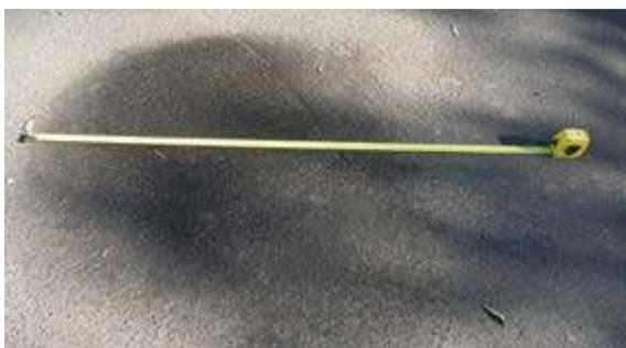
Step 2: Using water, on a dry surface, measure in metres the width of the spray pattern of the nozzle.
