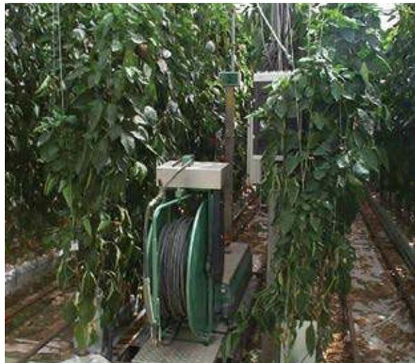
Above: Different makes of remote or unmanned sprayers are available that reduce exposure risks when spraying pesticides in greenhouses.
